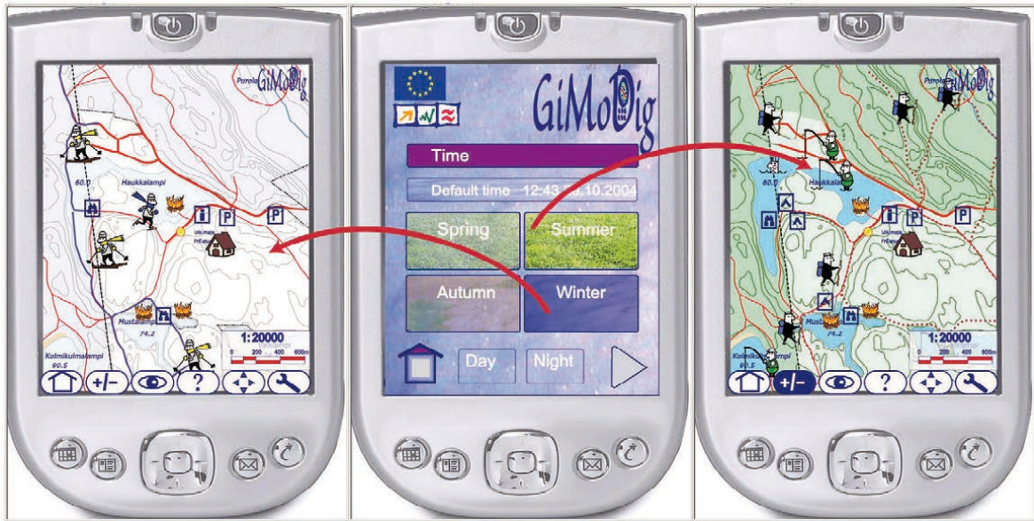
Fig. 2: Adaptive PDA maps for different seasons for the teenager user group. In the figure, three context parameters control the map: p_{TIME} \in \{ \text{"season:winter"}, \text{"season:summer"} \} , p_{AGE} = \text{"teenager"} , p_{DEVICE} = \text{"PDA"} . The context parameter p_{AGE} reflects to the choice of the style of the icons (for teenagers a comics style used). Depending on the context parameter value for p_{TIME} the delivered map has different contents and colours defined by the map specification modifiers.
