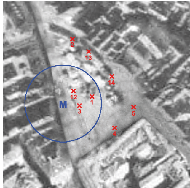
Fig. 3: Geo-Context, e.g., from GPS based position estimates ('M' with blue uncertainty radius), can set priors by geographically indexing into a number of object hypotheses ('X's are coordinates of user positions while capturing images about objects of interest).
