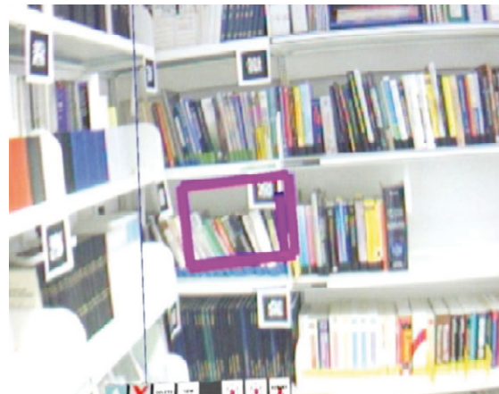
Fig. 8: The "Augmented Library" allows a user to quickly locate the shelf on which a book of interest can be found, by emphasizing the relevant location.
