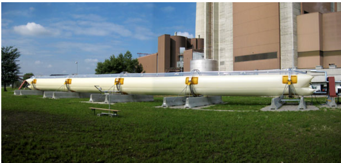
Figure 1.3: HELIOtube - A 40m inflatable trough concentrator in northern Austria, photo courtesy of Heliovis AG.
