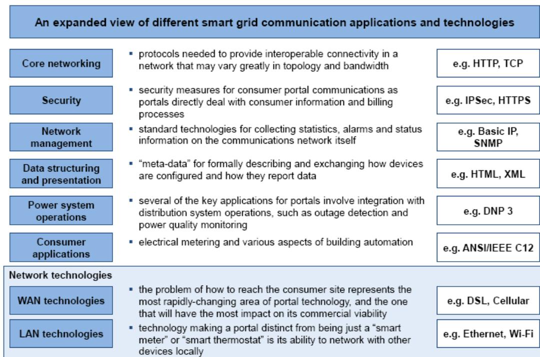
Figure 15 Overview of Smart Grid communication applications & technologies<sup>36</sup>
