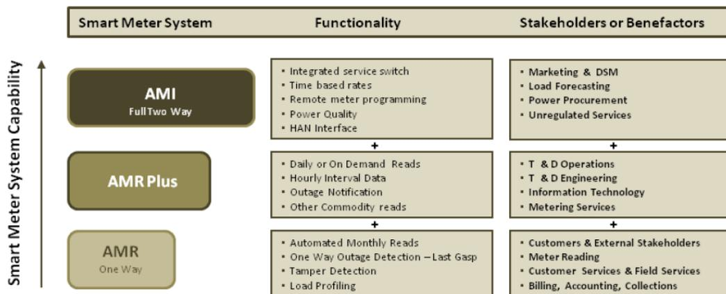
Figure 18 Smart meter technology evolution <sup>56</sup>
