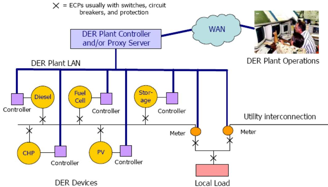
**Figure 19 Example of the communication and control of a DER plant**<sup>66</sup>
