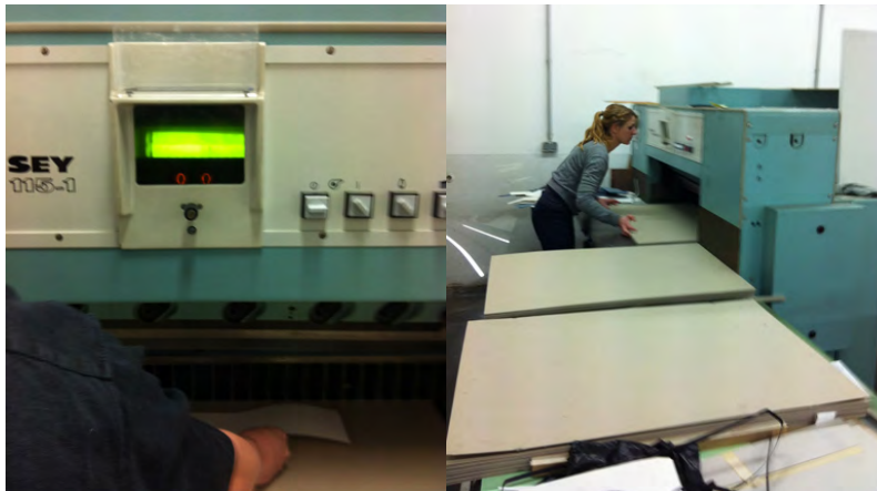
Fig. 3.70 The paper cutting machine programmed to cut strips of 9 cm and capable to cut six sheets of cardboard at a time.
