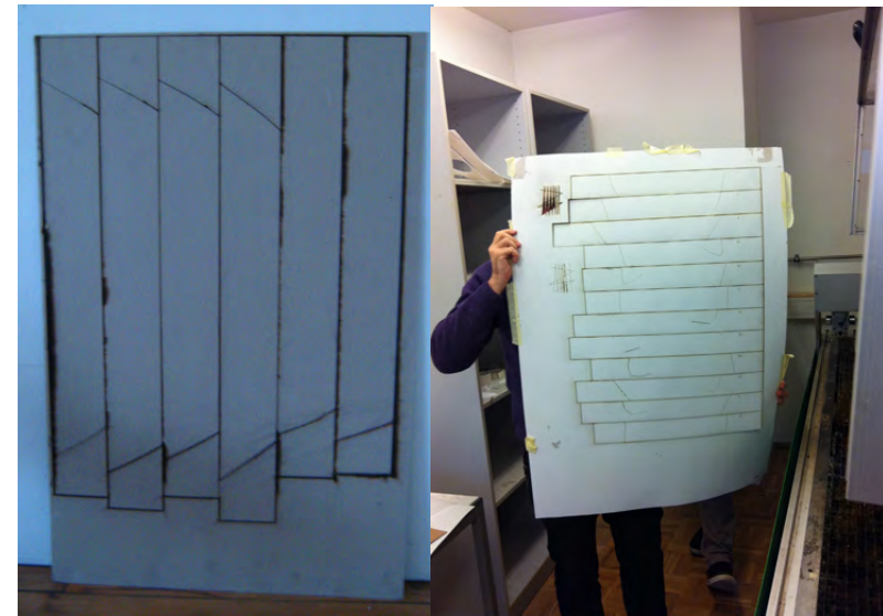
Fig. 3.66 A 2 mm sheet of cardboard sheet engraved (left); a 1mm sheet of cardboard laser-cut (right).
