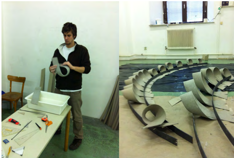
Fig. 3.72 Soaking the strips and criss-crossing the flaps (left); components drying (right).
