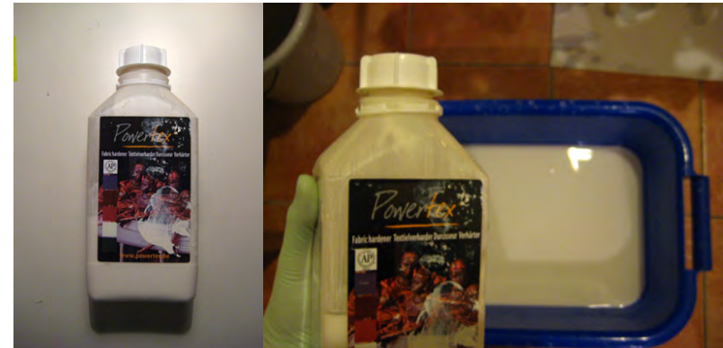
Fig. 3.21 Powertex bottle (left). Basin of water with textile hardener solution in which different paper, foam and textile materials are soaked.
