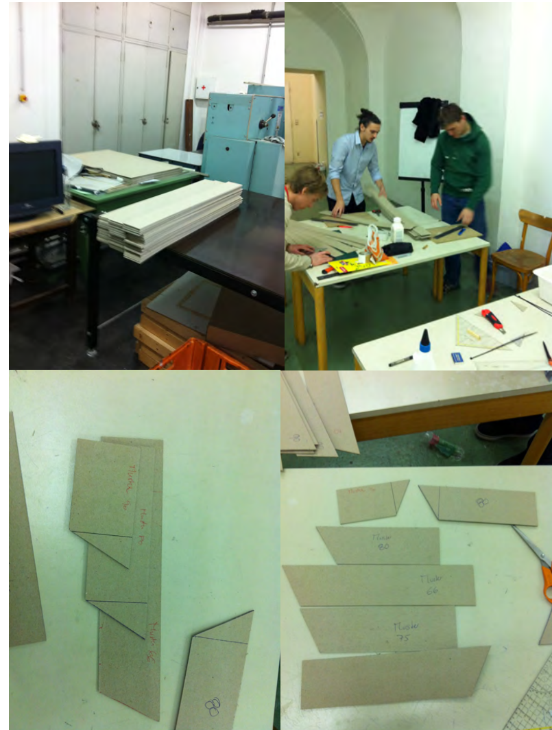
Fig. 3.71 Strips cut by the paper cutting machine (top left); cutting the strips at different lengths (top right). Helping templates for cutting the strips (bottom).
