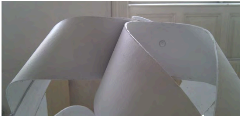
Fig. 3.51 Module joined with rivets and painted with spray paint.
