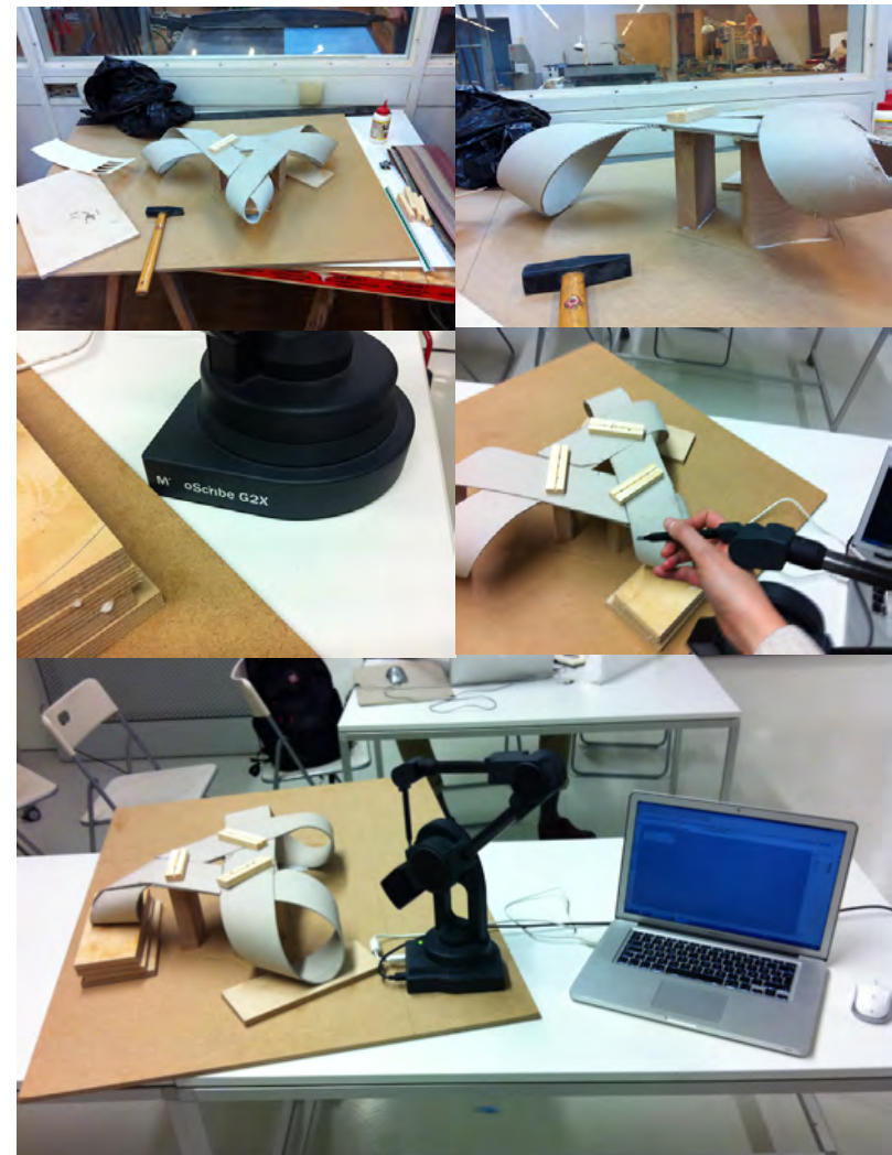
Fig. 3.60 One face of a module fixed on a wooden board (top). Digitizing the exact curvature of the strips (middle and bottom).
