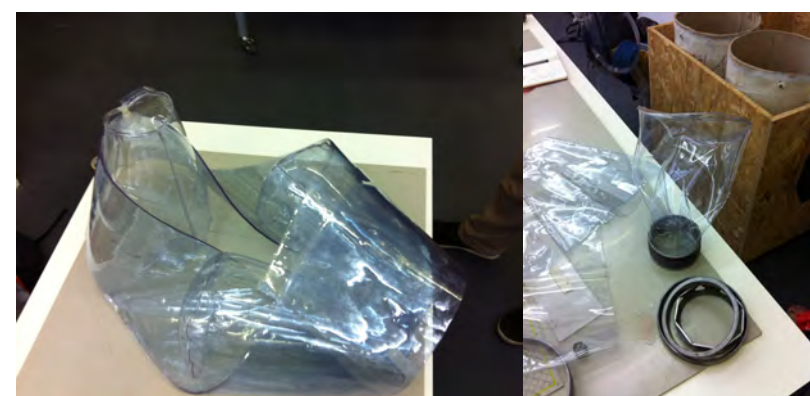
Fig. 3.26 Three conical shaped molds for keeping the cement shape in place (left); one conical shape in production (right).
