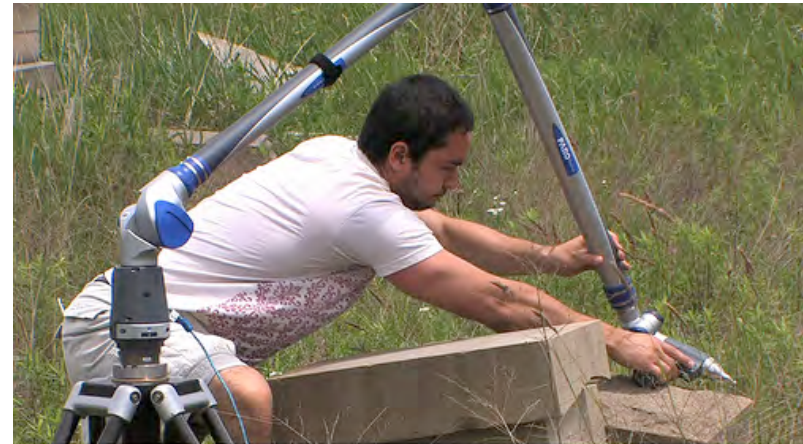
Fig. 2.21 Scanning scrap with portable outdoor scanning technology.
