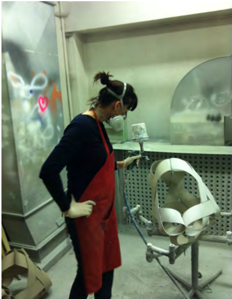
Fig. 3.78 Spray-painting of modules.
