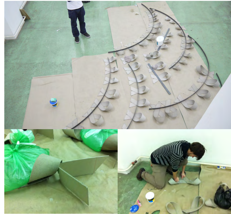
Fig. 3.73 Components drying (top); holding the components up with strips of cardboard (bottom left); glueing process (bottom right).
