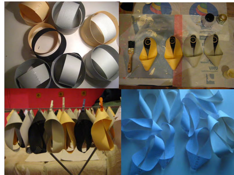
Fig. 3.28 Stapled loops out of thick paper strips (top left). Component kept intact after drying with the help of tea cups (top right). Components drying (bottom left). Shape of components after drying (bottom right).
