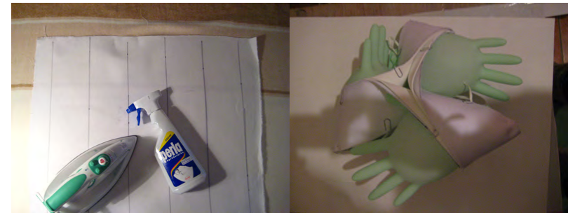
Fig. 3.25 Textile sprayed with a textile strengthening solution used for shirts (left). Textile soaked in hardener held by foam rubber molds and balloons (right).
