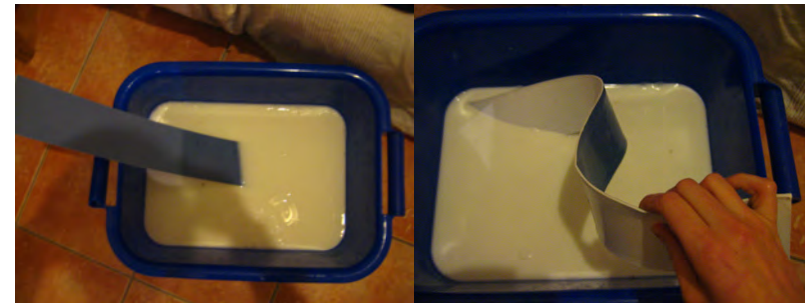
Fig. 3.35 Layered cardboard soaked in water and textile hardener solution.
