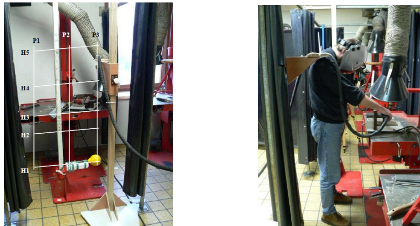
Figure 7-2 (left) Exposure setup for the MIG welding application with indicated measurement grid, and (right) typical position of the welder (Molla-Djafari et al, 2008)
