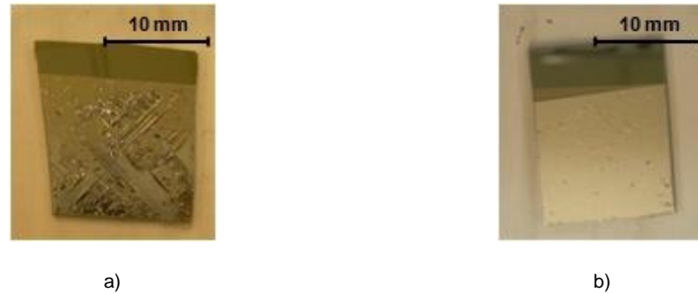
Figure 4.103 Images of AlCuFeB coatings with a Ni interlayer a) 200 nm Ni b) 1 \mu\text{m} Ni
