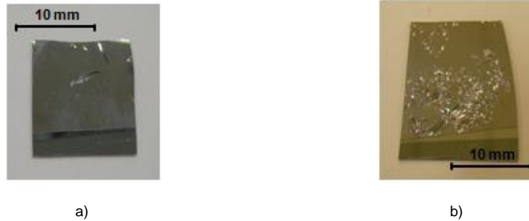
Figure 4.100 Images of AlCuFeB coatings with a Mn interlayer a) 200 nm Mn b) 1 \mu\text{m} Mn
