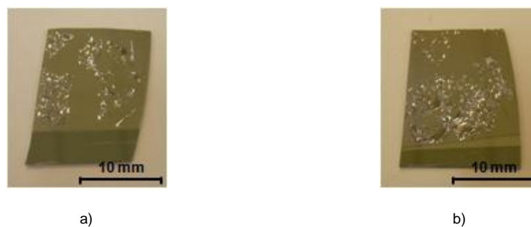
Figure 4.90 Images of AlCuFeB coatings with a Cr interlayer a) 200 nm Cr b) 1 \mu\text{m} Cr
