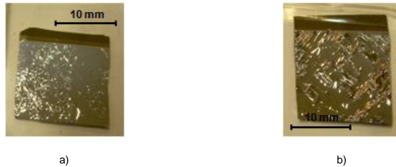
Figure 4.97 Images of AlCuFeB coatings with a Ti interlayer a) 200 nm Ti b) 1 \mu\text{m} Ti
