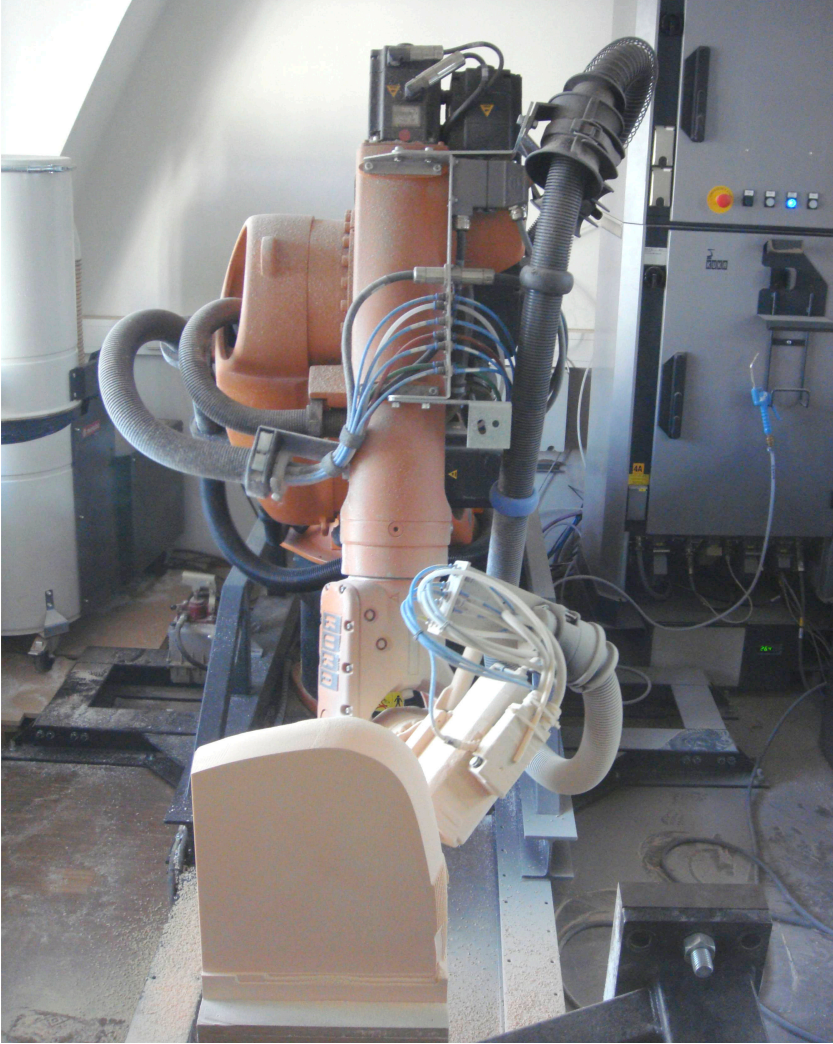
Figure 4.33 KUKA robot used as a milling machine at the Vienna University of Technology (2008).
