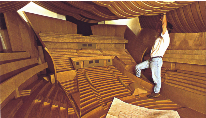
Figure 4.9 Acoustical study model of the Walt Disney Concert Hall, scale 1:10 (Gehry, 2001, p. 192).
