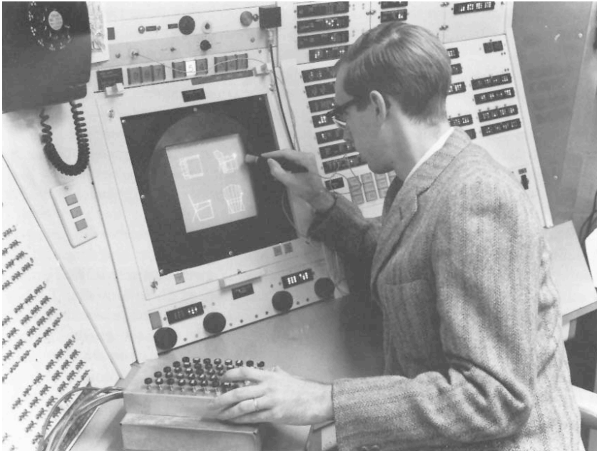
Figure 3.2 The Sketchpad developed by Ivan Sutherland in 1963 uses a light-pen to interact with objects on the screen (Schwarz, 1997, p. 61).
