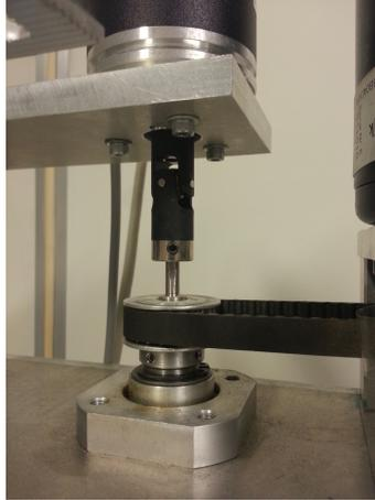
**Figure 6.1:** Rotary encoder sensor
