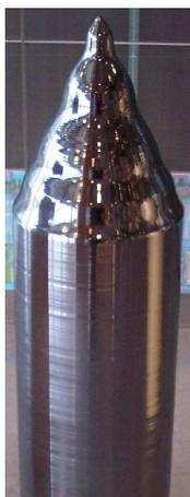
**Figure 4.23.:** A single-crystalline silicon ingot.
