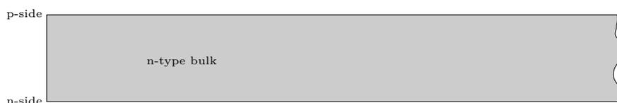
The processing starts with a n-type wafer (grey), which is thinned and polished by third-party wafer suppliers. An eventual p-spray implantation is carried out first, if n-side strip insulation is not achieved via the p-stop method. See section 7 for more information about these insulation methods.
