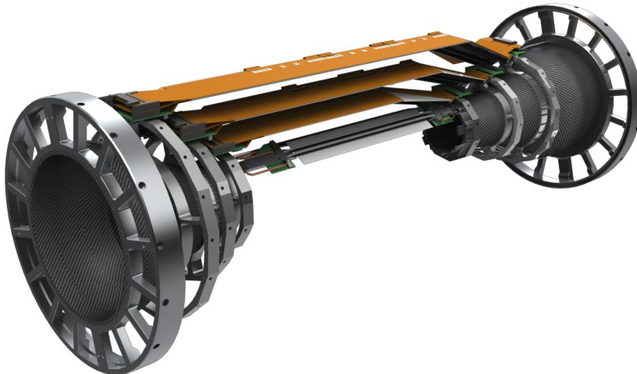
**Figure 2.6.:** Rendering of the support structure including the end flanges.
