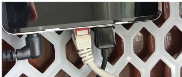
Figure 4.1: Loose contacts of a network cable (white)
