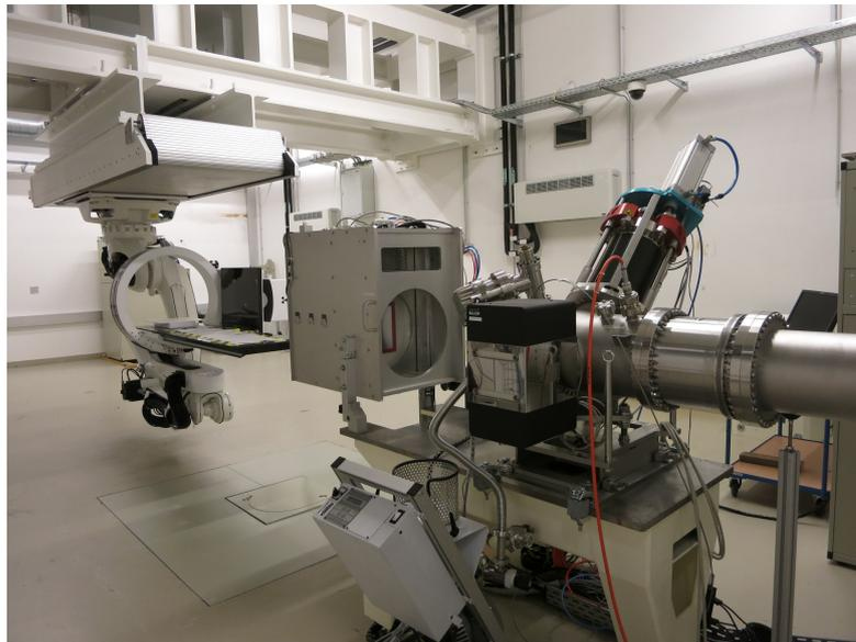
Figure A.4.: View of the robotic table in Irradiation Room 1 of MedAustron, for non-clinical research. The beam line on the right connects to the extraction line in the accelerator complex [44].
