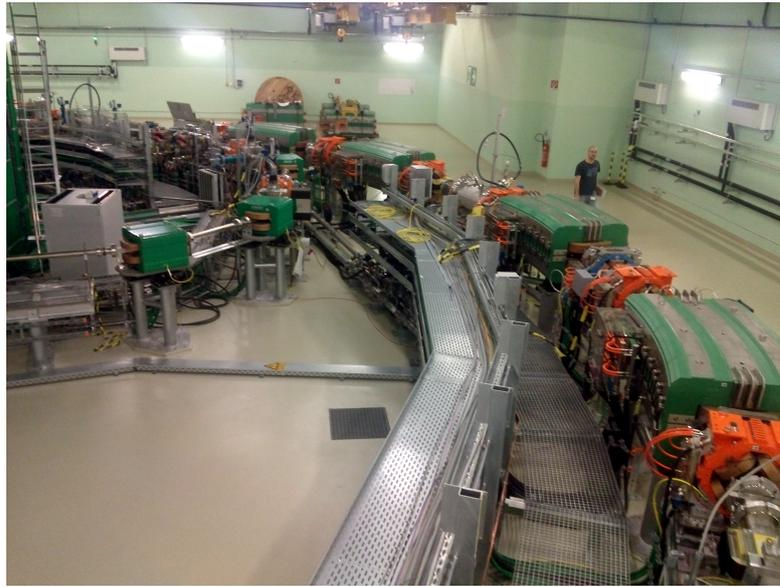
Figure A.3.: Photograph of parts of the accelerator at MedAustron, including the injection line at the left and a segment of the synchrotron ring at the right.
