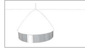
Then the rafters will be fastened at the end of the central pillar and supported by an umbrella-like structure. At last the roof will be thatched with grass. On the inside, the walls will be plastered with mud and straw
