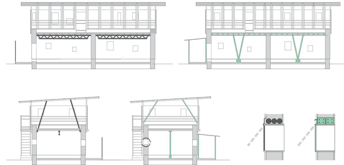
fig. 120: Changes from design (black) to construction (green) of the hostel building. Longitudinal- and cross sections M 1:200, section window M 1:100
