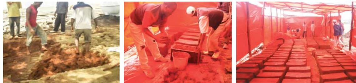
fig. 195: Mixing soil and straw
