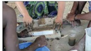
Another test is the linear shrinkage test. A mixture of soil and water will be pressed into a small formwork. When the material is dried out you can see the amount of shrinkage.
