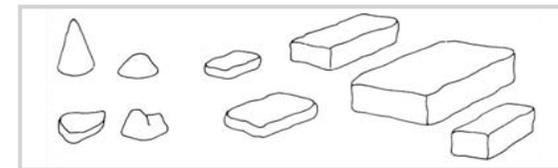
fig. 23: Different shapes of adobe bricks, made only by hand or with a mould
