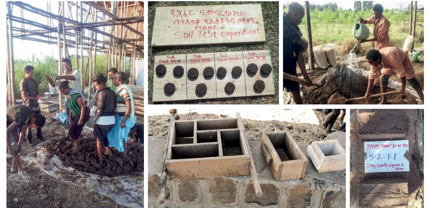
fig. 147: Soil inside mould
