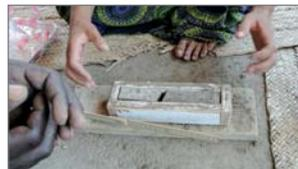
It becomes obvious that the sample shrank about one whole centimetre in length, which is a lot. Cracks are a result of this shrinkage, because when the sample gets smaller there is tension and it breaks.
