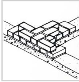
fig. 29: Bonding between walls
