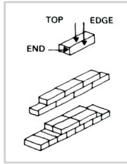
fig. 24: Surfaces of a brick, wall made of stretchers and wall made of headers and stretchers
