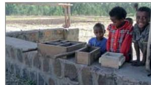
The mould has also been improved. Kafyalew Hailu (translated): "We wanted to increase the performance to safe time. So, I developed a new mould together with the town coordinator. With this mould, you can produce four bricks..."
