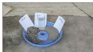
So, the components we need to produce adobe bricks are soil, sand and water. These components need to be mixed and soaked very well.
