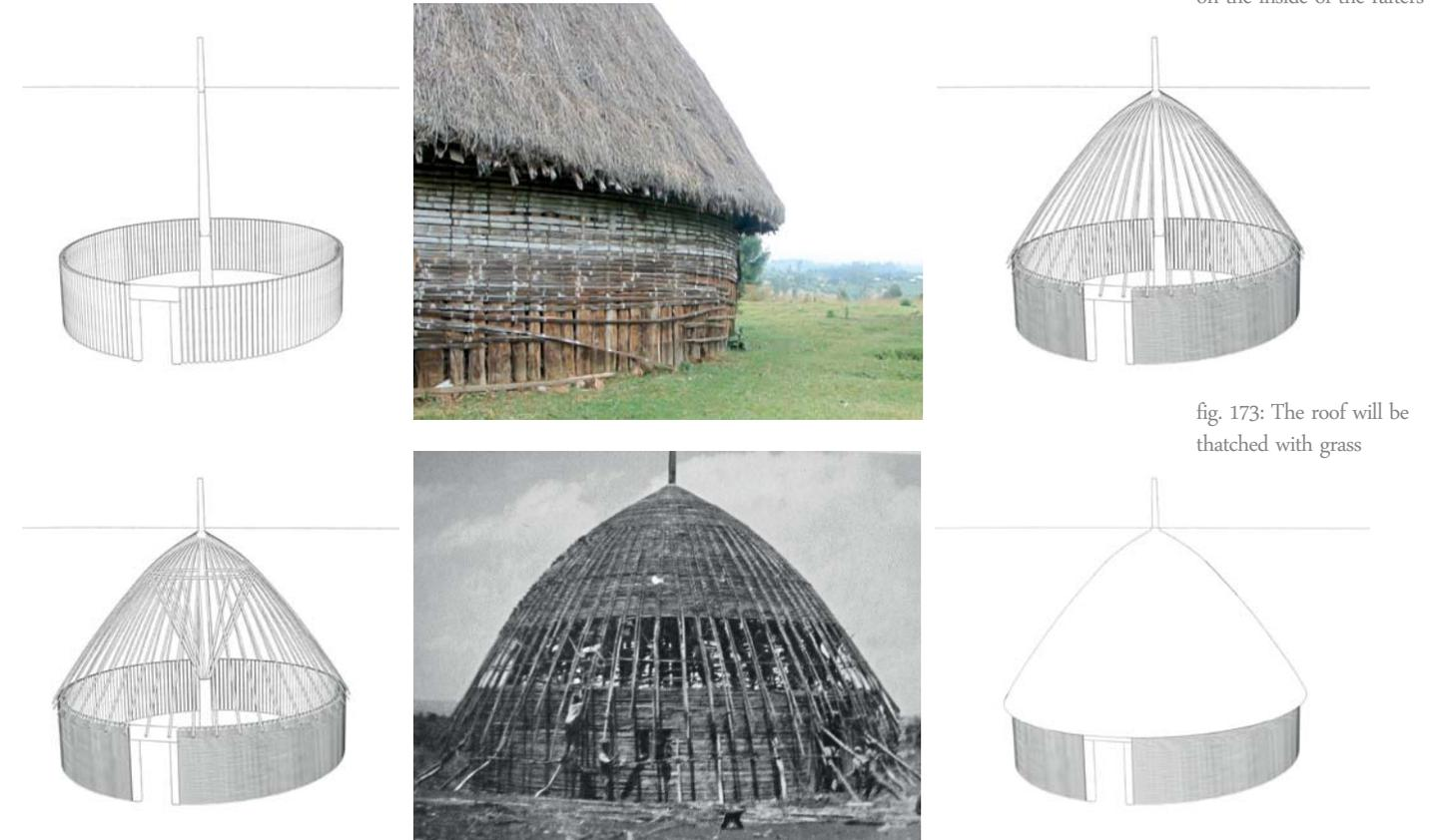
fig. 173: The roof will be thatched with grass
