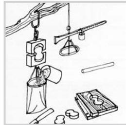
fig. 21: Binding force test on field
