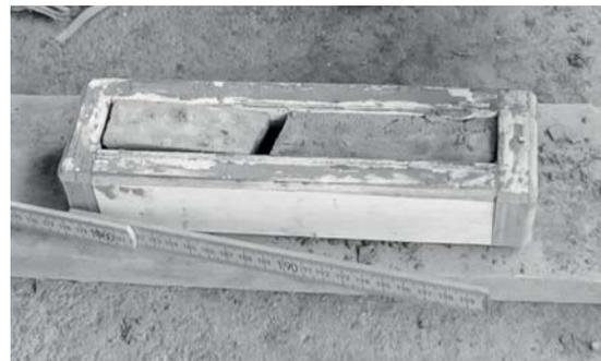
fig. 22: Linear shrinkage test carried out on the site of Afarkindergarten-project
