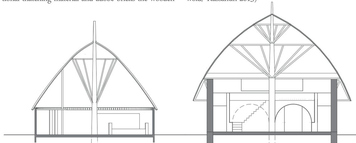
fig. 203: Section of a traditional Gurage house and SRDU M 1:200
