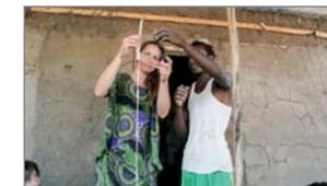
For the ball-dropping test you make a dry mixture of soil and water and form a ball with a diameter of about five centimetres. Then you let it fall from a height of about 1 metre fifty.
