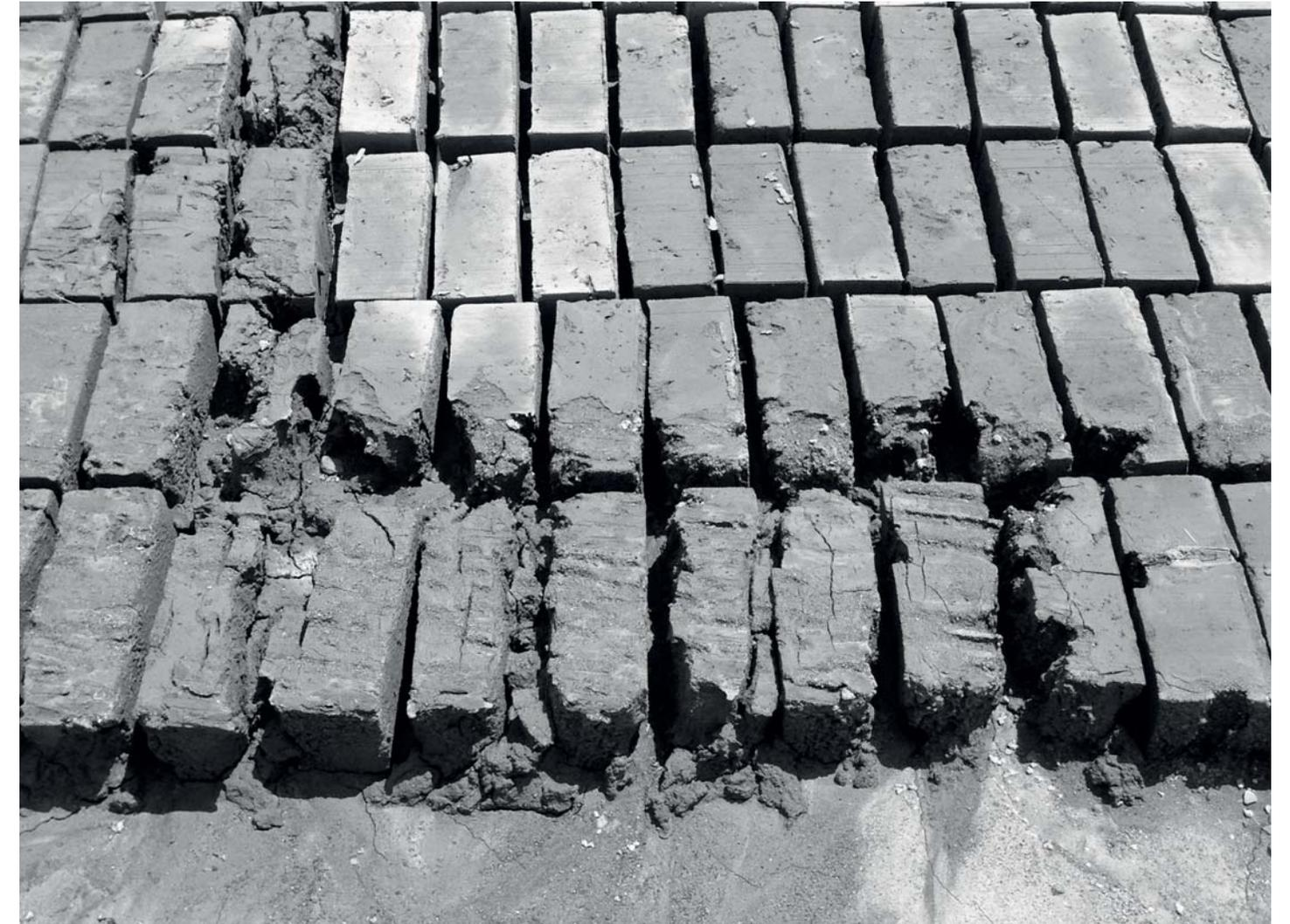
fig. 217: Bricks after rain
