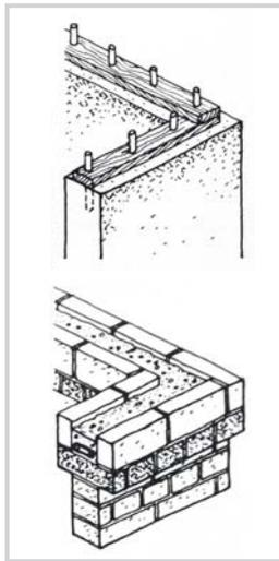
fig. 30: Ringbeam made of wood and reinforced concrete
