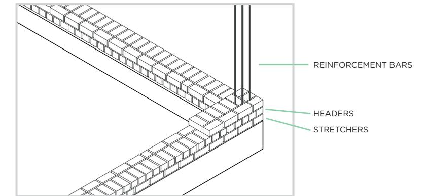
fig. 107: Brickwork of the hostel building M 1:50
