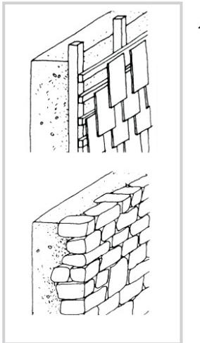
fig. 32: Coatings executed as covering or facing
