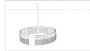
They traditionally live in round huts that have a characteristic construction. A central pillar will be erected first. Wooden studs dug into the earth form the wall. They are connected from outside, for instance with bamboo.
