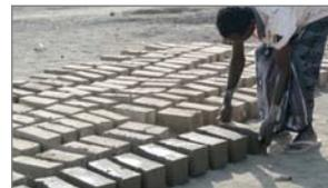
After one or two days the bricks can be carried outside and another one or two days later they will be stapled. About two weeks after production, they can be used for wall construction.
