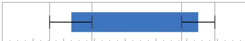
Figure 3.14: This is a bar visualization utilizing error bars to convey temporal uncertainty. The blue bar reaches from the mean start time to the mean end time of the visualized event. The black error bars denote the bounds of the two uncertainty intervals. [22]
