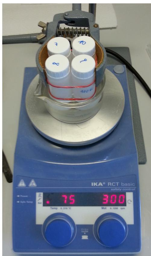
**Figure 3.7:** A metal clamp holds the four LSC bottles containing the  $\text{HNO}_3 + \text{H}_2\text{O}_2$  mixture and the TLD-600 dosimeters above a water bath. The bottles are dipped in far enough for the acidic mixture to be surrounded by water. The magnetic mixer is set to 75 °C and 300 rpm.
