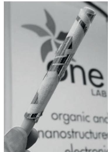
Fig. 2: Solar cells based on organic semiconducting inks integrated on top of fiber-glass fabrics. The flexible format of these solar cells allows them to be wrapped around a 5mm diameter object. Such devices can appear as lightweight curtains which are capable of producing between 40 and 100 Watts of electrical power per square meter, when exposed to standard AM1.5 solar illumination.
