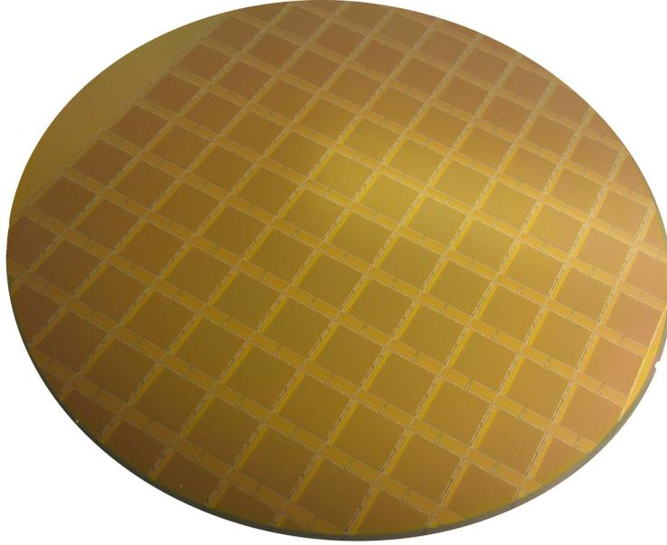
Figure 3.4: Picture of one readout wafer containing 86 ALICE1LHCB readout chips.
