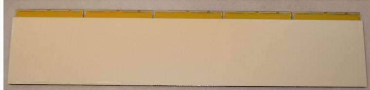
Figure 3.2: Picture of one ALICE SPD ladder. 5 ALICE1LHCB readout chips flip-chip bonded to one silicon sensor are visible. The silicon sensor has full aluminum back-side metalization (see chapter 3.2.2)
