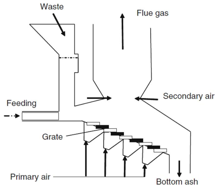
Figure II.2: Schematic drawing of a grate-based combustion system for MSW. Source: [Spl10]
