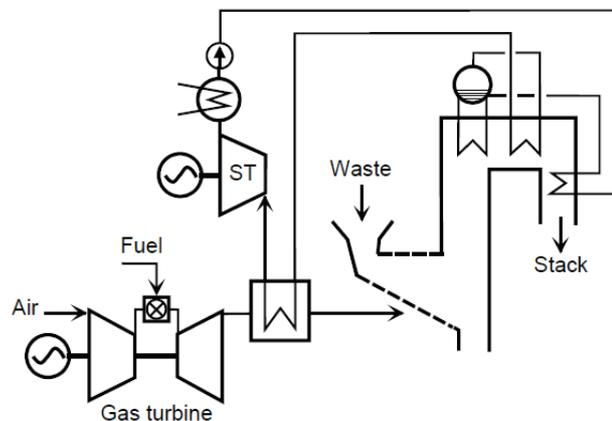
Figure II.3: The hot windbox configuration with superheating. Source: [Kor98]
