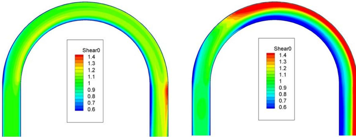
Figure 3.13: Distribution of bed shear stress at the beginning and the end of the run
