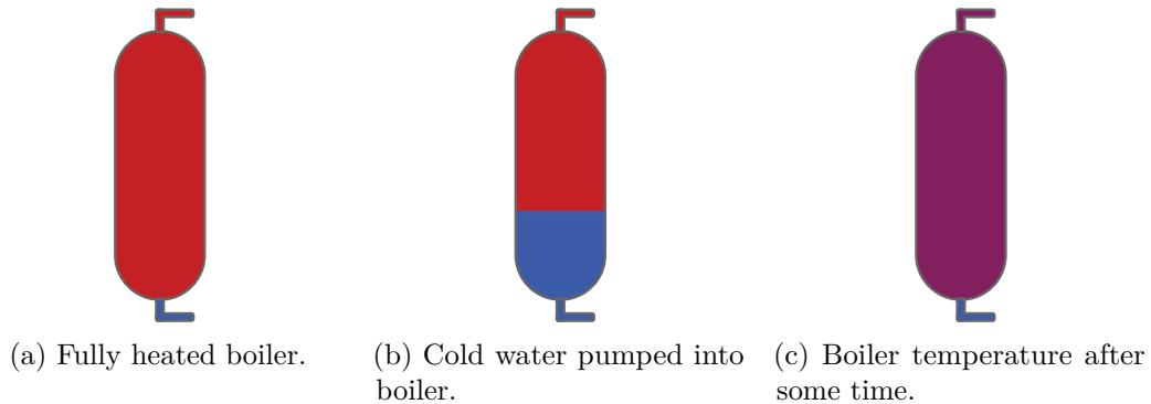
Figure 5.12: States of the boiler at the time of consumption.
