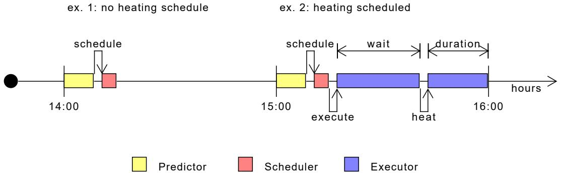
Figure 5.3: Examples of derived schedules and the execution thereof.
