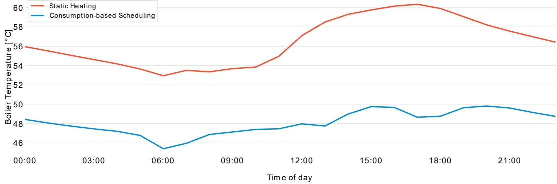
Figure 6.12: Boiler temperature before and after switching to consumption-oriented scheduling
