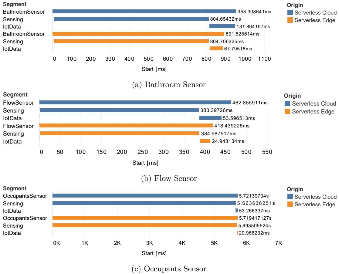
Figure 6.7: Execution Time of IoT devices
