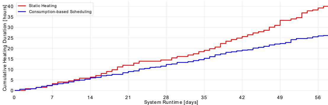
Figure 6.13: Heating time before and after switching to consumption-oriented scheduling
