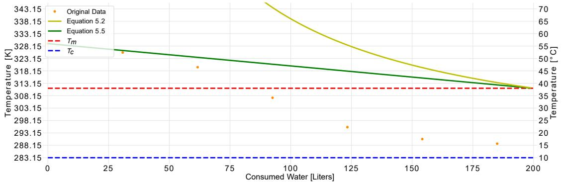
Figure 5.11: Boiler temperature when consuming warm water
