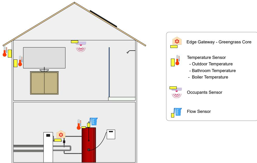
Figure 5.4: IoT devices installed in a home for *Elastic Heat*
