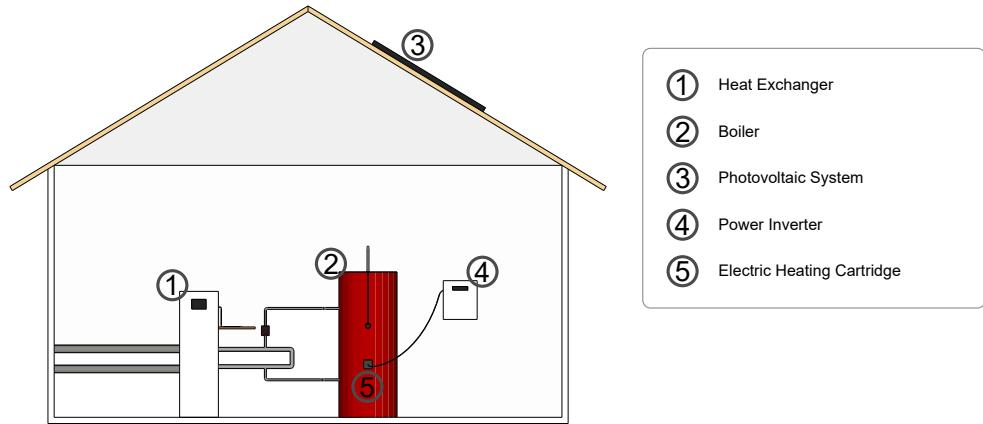
Figure 4.2: Home equipped with district heating and photovoltaic system
