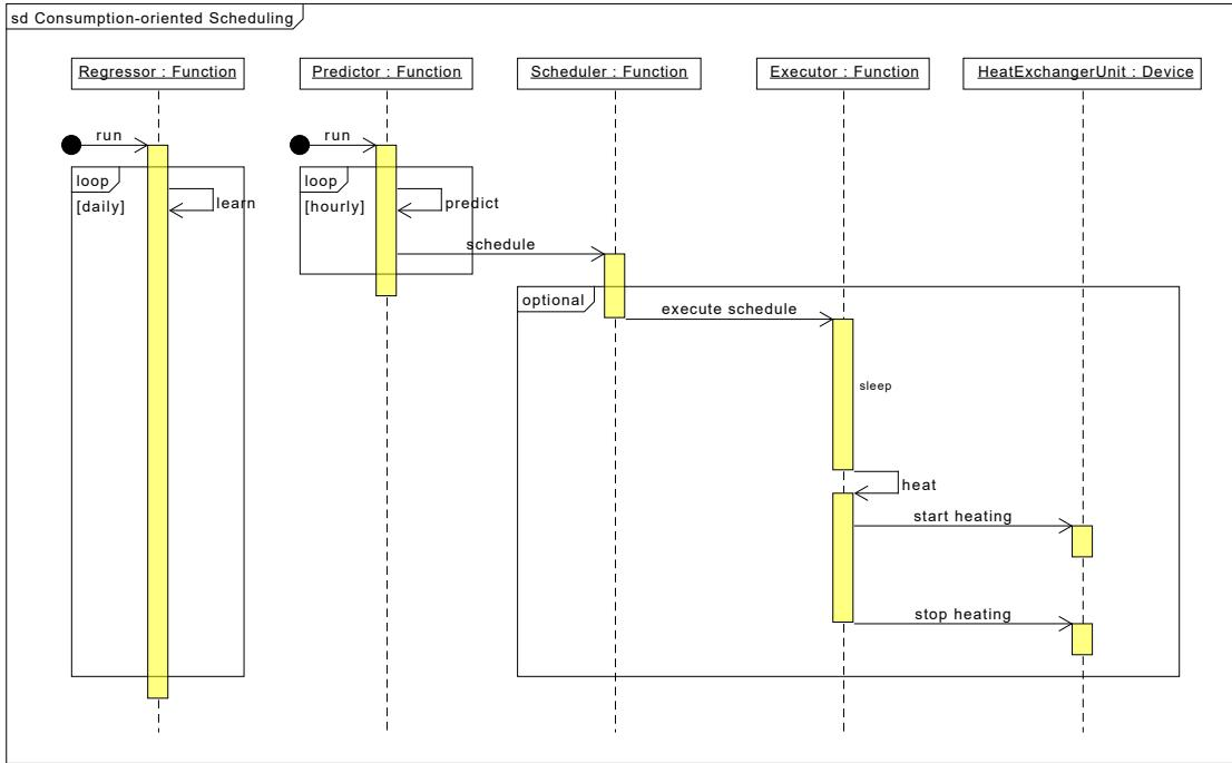
Figure 5.2: Scheduling Process Flow of *Elastic Heat* components/functions
