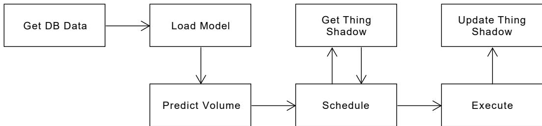
Figure 6.6: Execution flow of Predictor function including scheduling and execution
