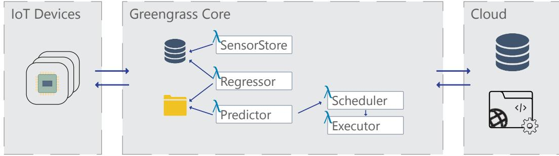
Figure 5.1: Fundamental architecture of a serverless predictive analytics platform at the edge. Implemented in *Elastic Heat*.
