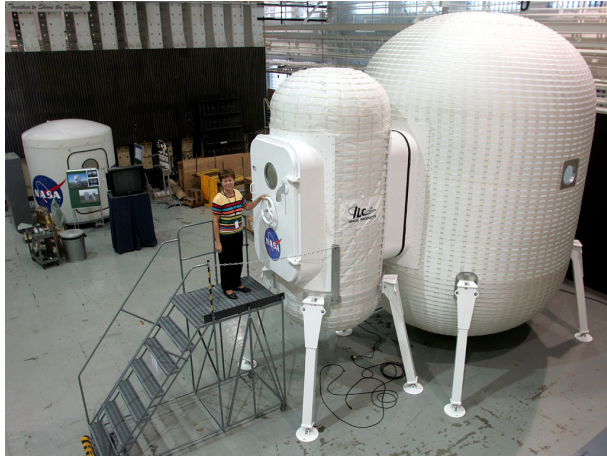
Planetary Surface Habitat with Airlock Mock-up Unit from 2007. Credit NASA/ ILC Dover
