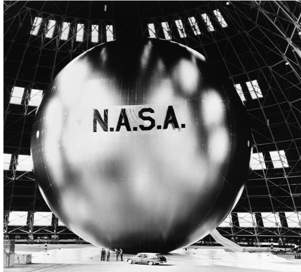
Echo Satellite Inflation test 1961, Diameter 31m Credit: NASA
