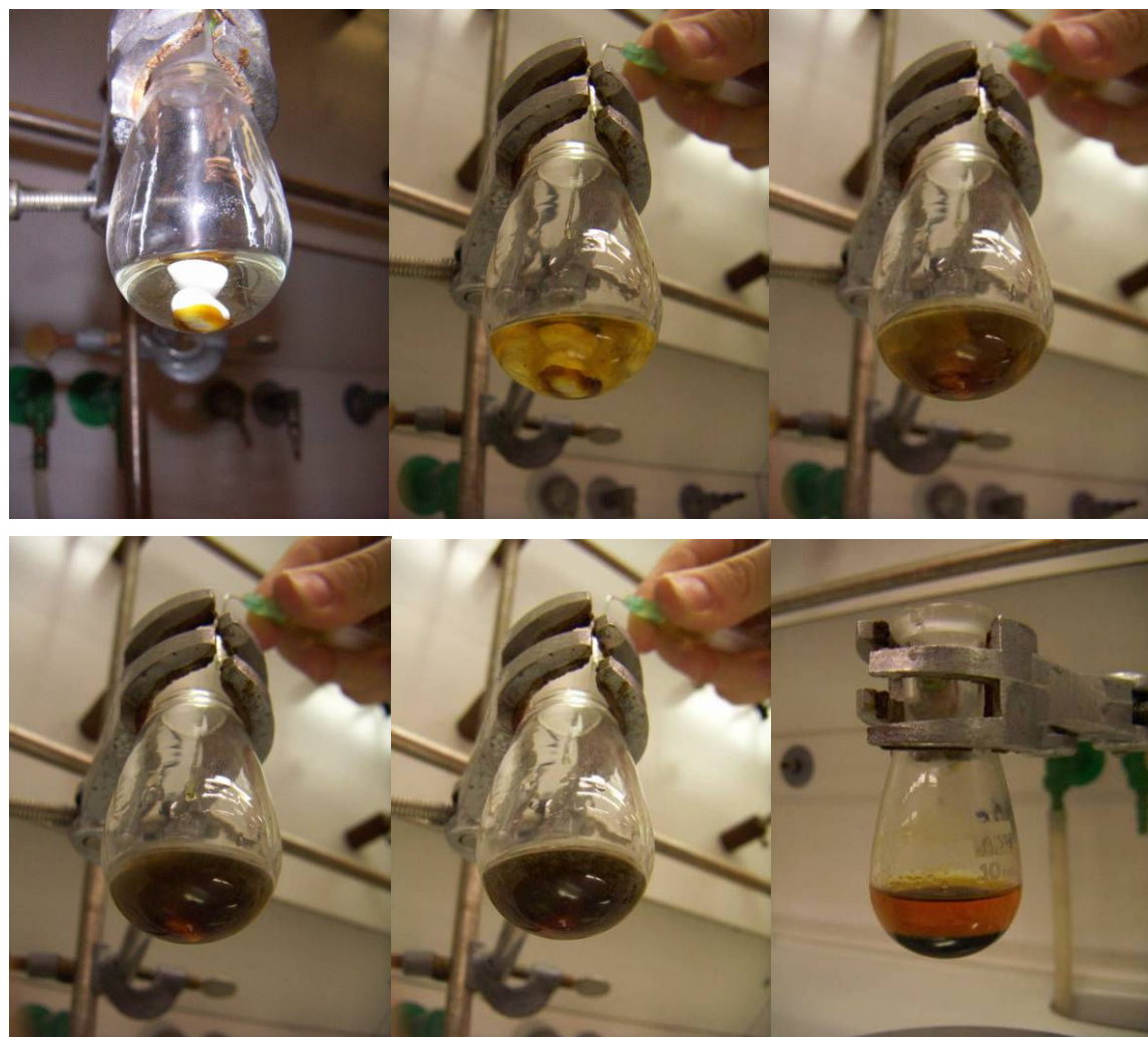
Figure 70: Progress of the addition of 4-fluorophenylmagnesium bromide to the biphasic reaction mixture
