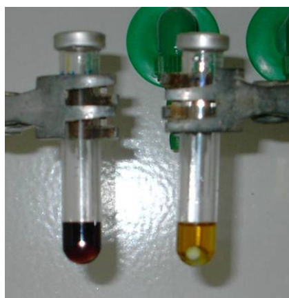
Figure 73: Fe(III)-ato complex of bmim-FeCl 4 55 and methyl 2-oxocyclopentane carboxylate 81 and colour change observed after complete conversion.
