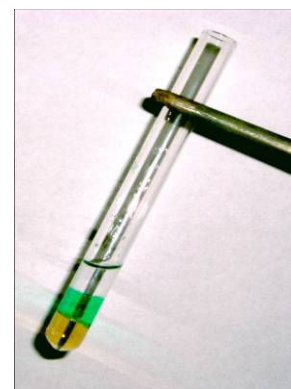
Figure 21: Triple-phase system of n -hexane (upper layer), water (dyed with \text{Ni}^{2+} ) and CIL 4c (lower layer)
