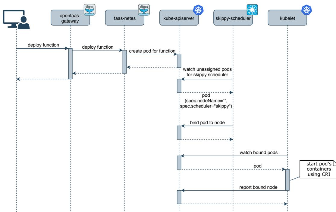
Figure 5.3: Sequence diagram of a function deployment
