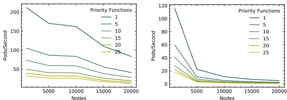
(a) Scheduling throughput when using the default algorithm (b) Scheduling throughput when scoring all available nodes
