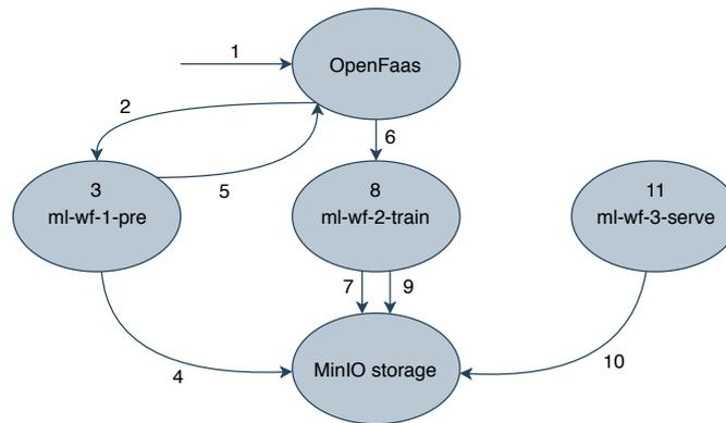
Figure 4.6: Execution-graph of a single workflow execution
