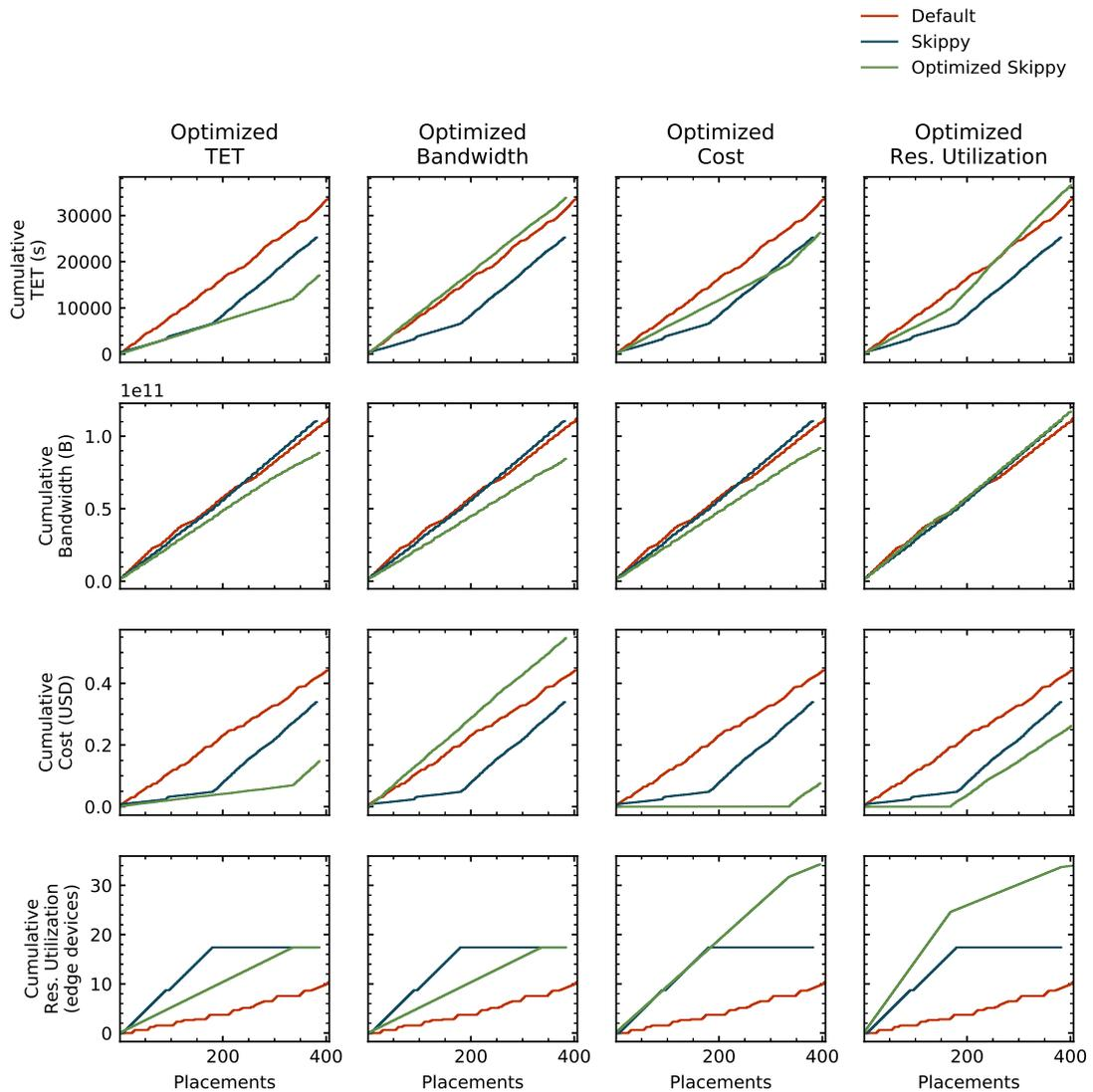
Figure 7.6: Placement quality comparison matrix plot for the *cloud\_100* cluster configuration
