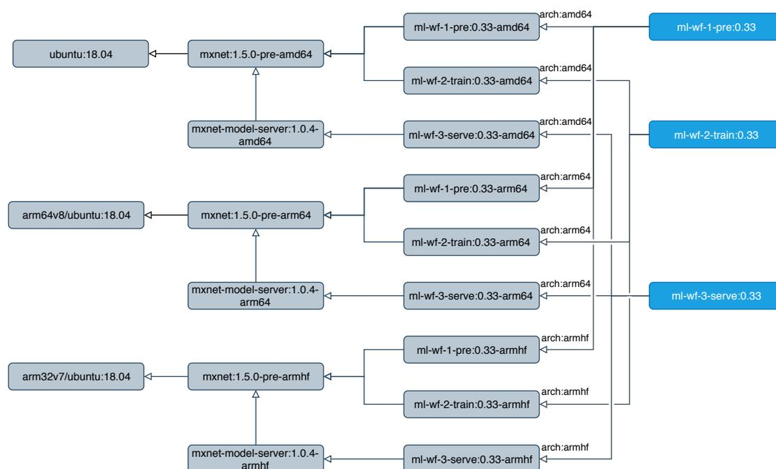
Figure 4.7: Hierarchy diagram of the workflow function Docker images
