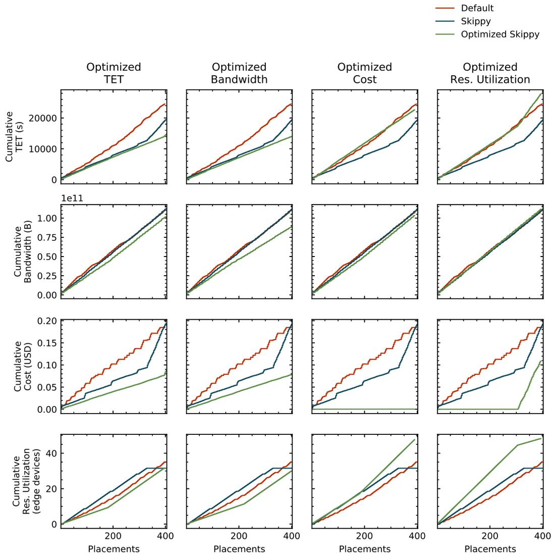
Figure 7.9: Placement quality comparison matrix plot for the *edge\_100* cluster configuration
