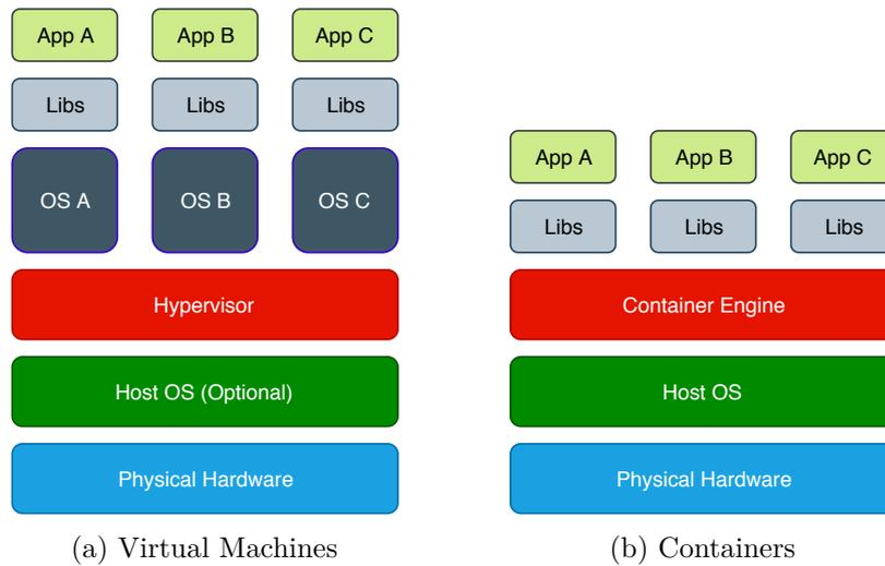
Figure 2.4: Architectural comparison between virtual machines and containers according to Bernstein [Ber14]
