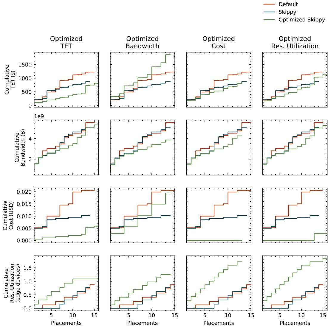
Figure D.1: Placement quality comparison matrix plot for the *testbed* cluster configuration
