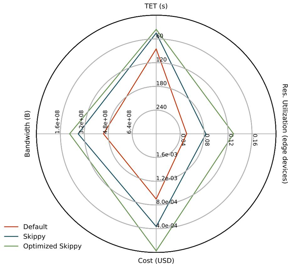
Figure 7.12: Mean values for each objective over all simulated experiments per scheduler
