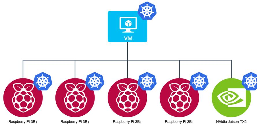
Figure 4.2: Illustration of the nodes in the testbed
