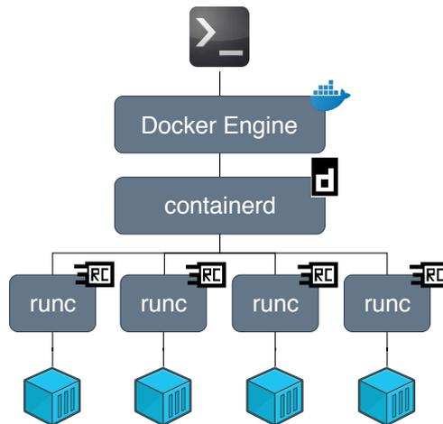
Figure 2.5: Docker architecture: The user interacts with the *Docker Engine*, either by using the Docker CLI or via other tools like a container orchestrator. The Docker Engine instructs *containerd* to create the container. *containerd* is then using *runC* (or any other OCI compliant runtime) to actually spawn the container, whose library *libcontainer* in turn is then finally using the kernel’s API.
