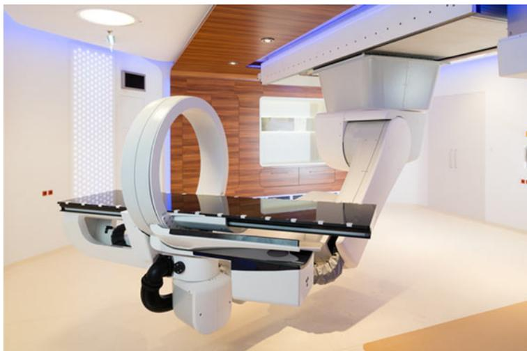
Figure 2.1: ImagingRing™ System at MedAustron (from [43]) The ring surrounds the patient couch. Both are mounted on a robotic arm. X-ray head and detector are positioned underneath the patient couch.
