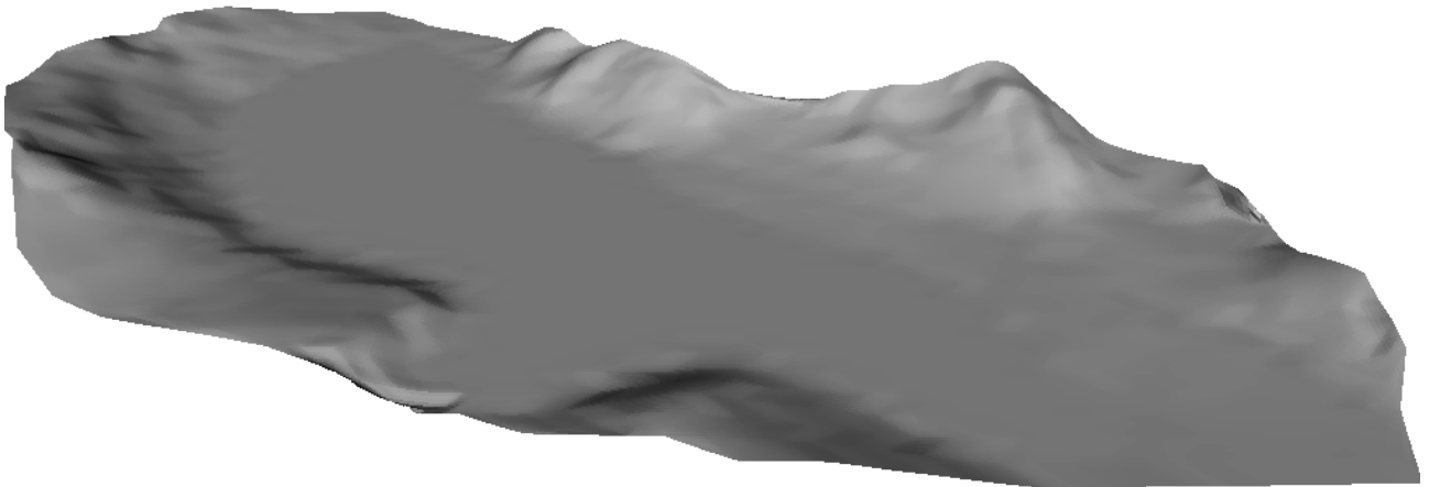
Figure 6.12: Gently sloping terrain surface reconstructed with an interpolating/approximating subdivision approach based on paraboloids as local surfaces.
